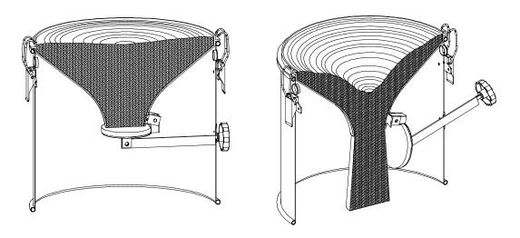
For opening flap, loose star knob (2-3 rotations) and hold it up slightly. The reusable or new blast grain will get into the jet material container (lower container). Hold the star knob up and press it in direction of container again for closing the flap. Tighten star knob.
