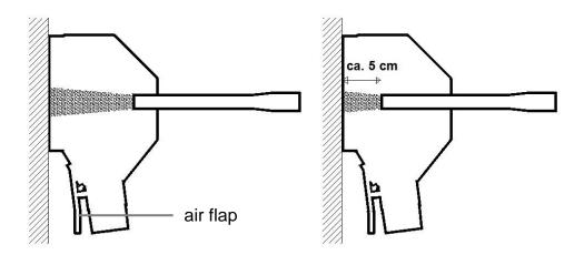
**Note:** Tilt the jet hood at the top first, so that residues of blasting media are collected and sucked off.
